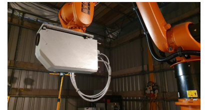
Robotized LUS-system with fiberized scan-head for aerospace applications
